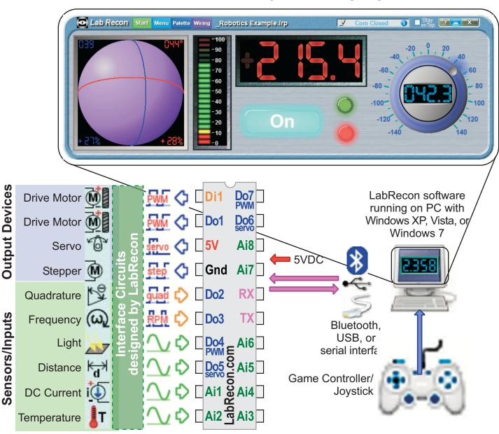
Sensors, such as for light and distance can source values on the Panel and can further be used to control the outputs by creating control logic on the Wiring Diagram.
