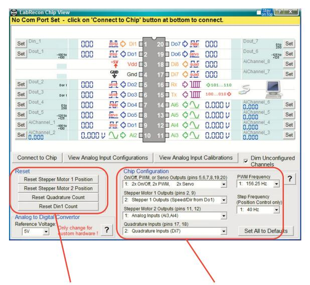
These buttons reset the counters associated with the Stepper Motor Outputs, the Di1 Counter, and the Quadrature Counter.
